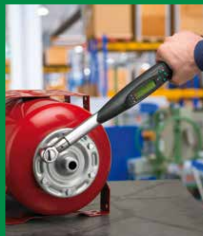
Example of static measurement with digital dynamometric wrench
