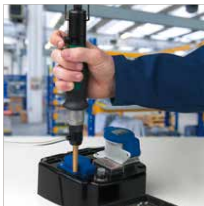
Customised screwdriver with suction device useful in case of non-magnetisable stainless steel screws
